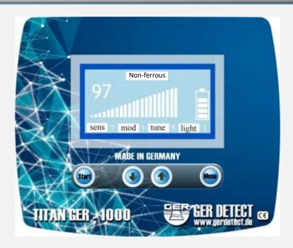
Adjust the sensitivity by the navigation buttons UP & DOWN.
