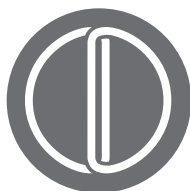
The strongest signal occurs where the Tx and Rx coil windings overlap.
