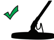
Correct search coil angle
