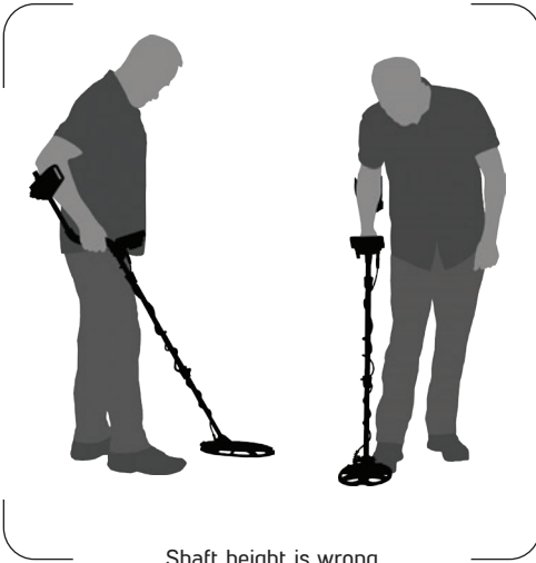
Shaft height is wrong
