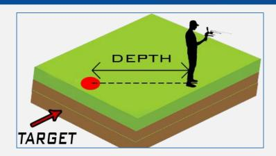
Measure the distance between the antennas reversing back and the target center point.
