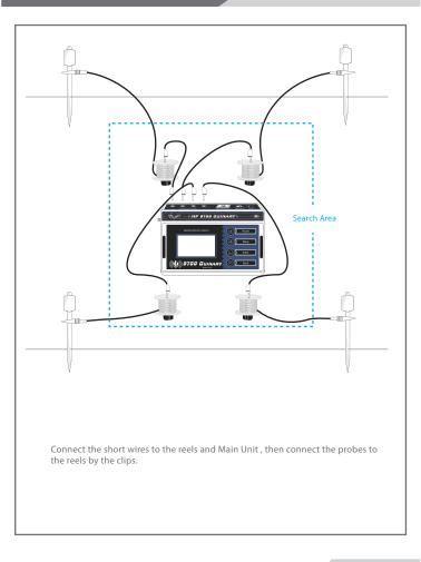
2- Make sure that the distance between the probes is equal If -for example- the distance between probe 1 and 2 was 15 meters the other probes should be distanced at the same length which will form a square as shown in the figure below.
