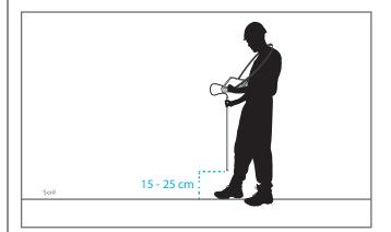
Before starting the user has to balance the device and adjust the sensitivity according to the ground by pressing ENTER or the Button on the top of the Ground Sensor to take a balancing measurement in a stable place unaffected.
