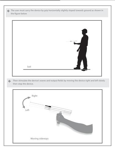
In the case of a located target , the device will receive signal and a reading that will divert the device from the normal track to another track which is the target point track,
