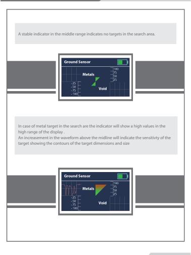
In this case the existing target is void and the interactive indicator with high values of blue according to the received signals and the target size in the search area A diffrential signals on the waveform will show the an increasment over the midline when cavity is sensed and the waveform would decrease below the midline after passing the target which will give the user an estimation of the cavity or void size and dimensions.
