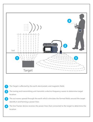
If you selected the Line Tracking search method, make sure that the Line Tracker is switched on and the indication LED is on then the Main Unit will send the start command to the Line Tracker with the selected parameters.
