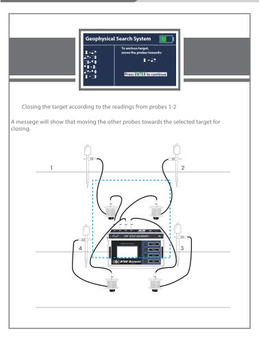
After moving the probes closer towards the probes (1-2) and pressing (Enter) the device will restart the scan process to confirm the target.
