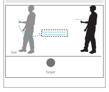
There is another way to locate the target point more accurately, (Square method) take 4 different readings for the target from 4 angles forming a square 3 m from target point the intersection point of the for readings is the target point.
