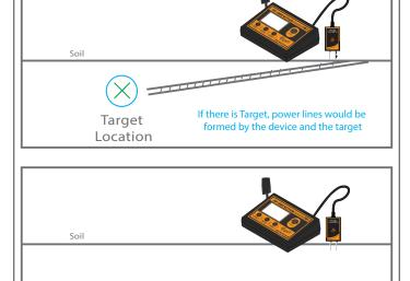
If there is no target the device would not form any power lines
