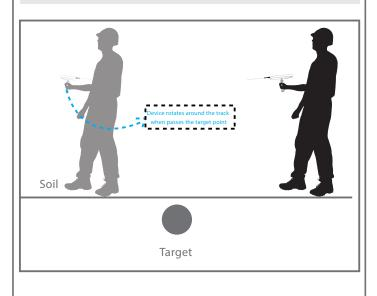
There is another way to locate the target point more accurately, (Square method) take 4 different readings for the target from 4 angles forming a square 3 m from target point the intersection point of the for readings is the target point.
