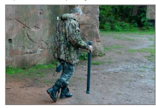
Push the button to start scanning the underground. Move the Super Sensor slowly from one side to another above the desired object. Try to capture the complete object, which means measure beyond the edges of the object. Repeat this measurement a few times to get a clear signature of the object. During this procedure the Super Sensor should point vertical towards the ground.
