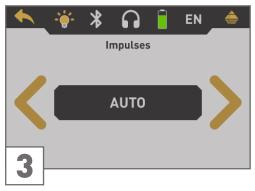
First, set the number of measure points (Impulses), which will be recorded for each single scan line.
