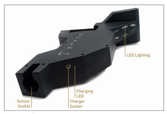
**Charger Socket / Charging LED:** When the internal battery is too low, you have to recharge it by connecting the appropriate charger to the Charger Socket. As long as charging is in progress, the Charging LED is **orange**. As soon as the Charging LED turns off, the battery is fully charged.
