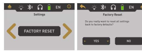
Use the > button to highlight the "Yes" option and push the **OK** button to start the factory reset. If you do not want to reset your device select the "No" option instead or push the button.
