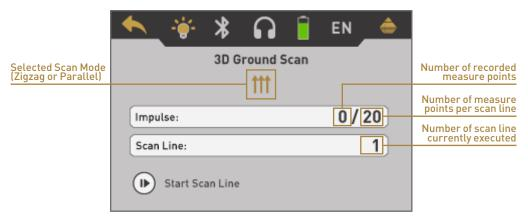
The display indicates that the first scan line has started and no impulse has been measured up to now. In total, there will be 20 measure points per scan line. The device is waiting for the user to press the button to begin the measurement recording.
