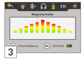
The display shows the active Magnetometer screen. You can repeat the ground balance at any time by pushing the button.
