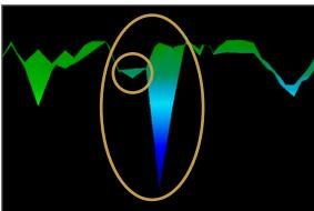
Another signature to look for is the one that is also commonly referred to as a "hit within a hit". The scan image needs to be viewed from the side view and fitted onto the screen. If the values are too high, you won't be able to recognize the differences.
