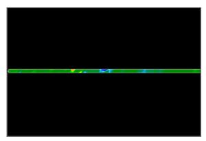
After transferring the scan data to Visualizer 3D Studio you will see a scan that is a straight line. This scan is now ready for analysis.
