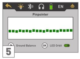
The display shows the active Pinpointer After canceling the Pinpointer mode, the descreen. You can repeat the ground balance at vice also exits the wireless data connection any time by pushing the button. The LED before returning back to the main menu. Orbit can be enabled by pushing the **OK** button. The visual representation on the screen is very rough and should not be used to distinquish the signatures.
