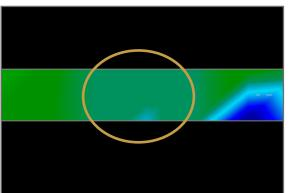
This scan shows the highlighted section of how a natural mineral field appears like. Please note the above colors, they are difficult to notice when in direct sun or bright light. Analyze your scan in an area where the computer can be shaded from most of the natural light to better recognize the colors.
