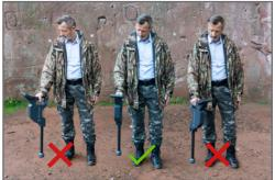
As soon as an acoustic signal sounds, the device has detected a potential metal target right under the position of the probe. In this way it is possible to find small metal objects near the surface like nails, screws, wires, seals and similar targets.
