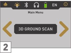
Probe is connected, confirm the operating mode "3D Ground Scan" by pushing the **OK** button.
