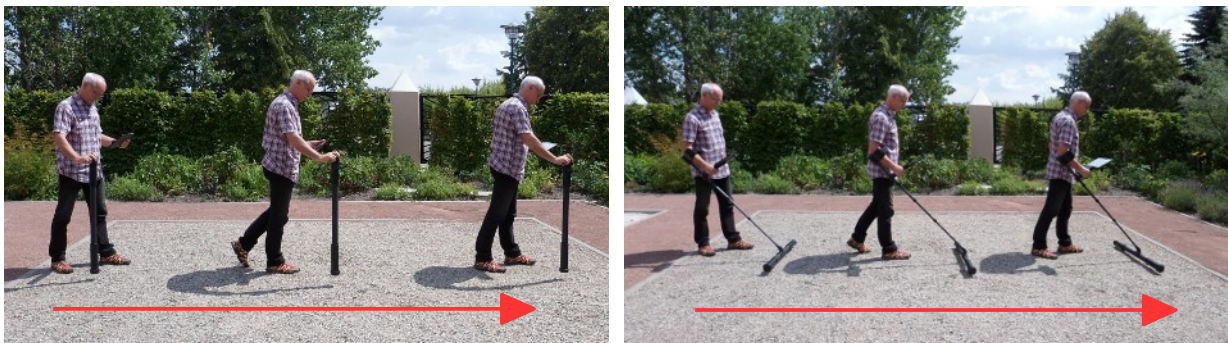
Figure 6.5: Ground Scan in vertical and horizontal mode
