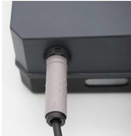
Figure 6.1: Connection of probe
