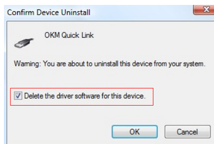
Figure 2.25: Uninstall USB drivers on Windows Vista, Step 2
