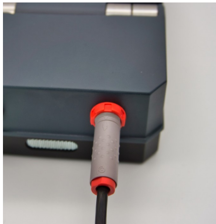
Figure 6.2: Connection of Power Pack
