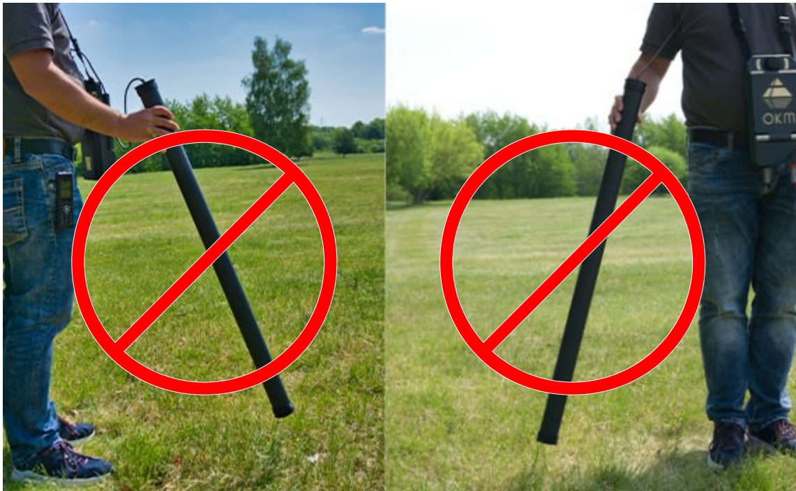
Figure 9.3: Super Sensor Wrong Orientation
