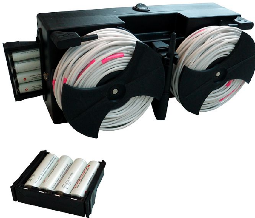
Figure 6.1: Placing batteries into the Controller's compartments
