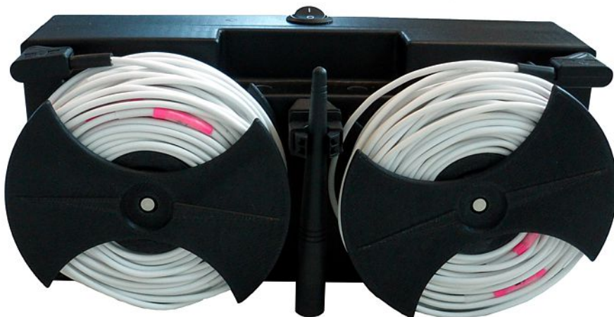
Figure 6.4: Voltage Cable Drums mounted to Controller
