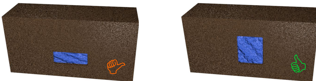
Figure 7.1: Detection of thick objects is better than flat objects
