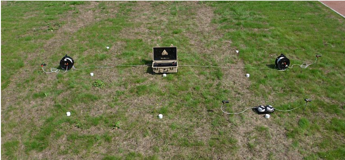
Figure 7.7: Arrangement of electrodes during Active Scan (Quick)
