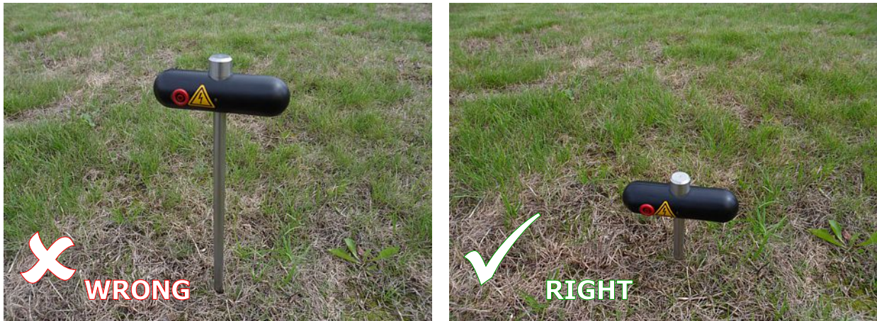
Figure 9.1: Electrodes need good electrical ground contact
