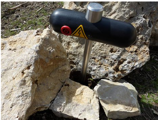
Figure 9.5: Drilling a hole and refilling it for the electrode
