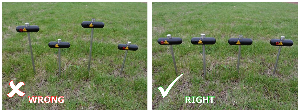
Figure 9.2: Electrodes have to be equally set into the ground
