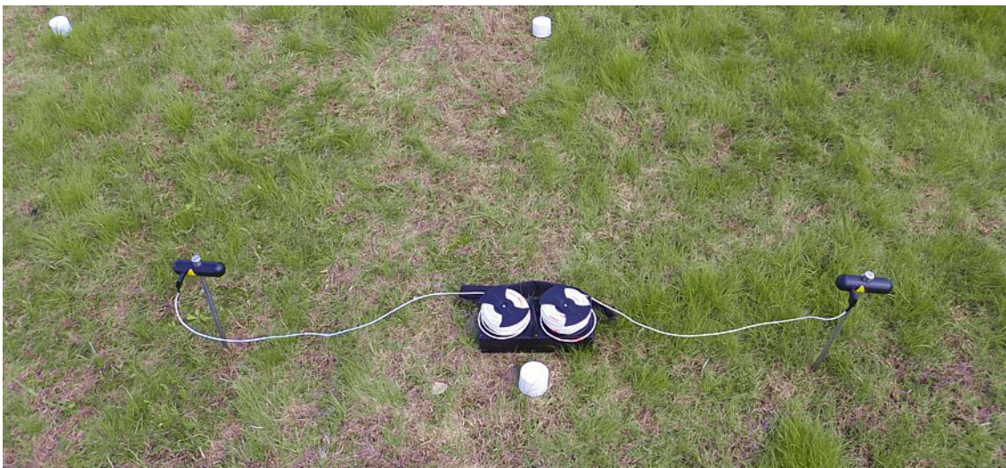
Figure 7.8: Arrangement of electrodes during Passive Scan
