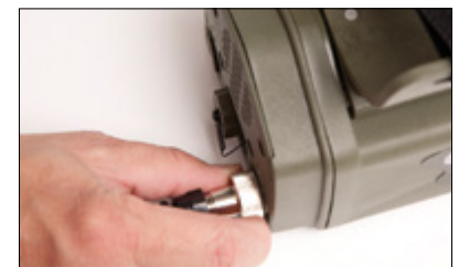
Hand-tighten connector collar.
