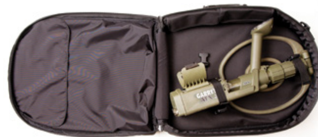
Figure 1: ATX with DD coil attached. Secure straps around lower stem nut and housing.
