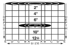
This object is larger than a coin, yet smaller than a 12-oz. can. It is buried at a depth of approximately 8"
